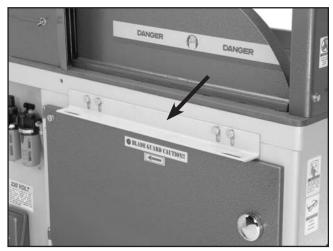
Figure 9. Mounting bracket attached to saw.
